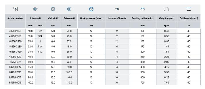
Vacuum resistance up to -0.5 bar (up to including 50mm ID), bigger sizes -0,3 bar
