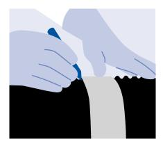
**1. MEASURING AND MARKING** Marking with a silver point pen; a metal sheet can be used as device or the half shells of the coupling can be placed provisionally on the hose.
