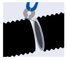
**3. PULLING THE STEEL WIRE HELIX** Pull the hose halves apart; pull the steel wire helix from the cut surface and cut it with a hack-saw or cable cutter at the center of the hose – the spiral must never tower above the cut surface and must not stick out of the rubber!
